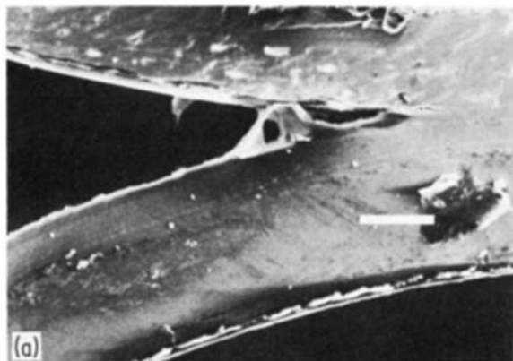
Figure 7 Partial removal of surface layers from the lower PET strip: (a) before breakage of ligaments; (b) after breakage. Scale bars 30\ \mu\text{m} .
