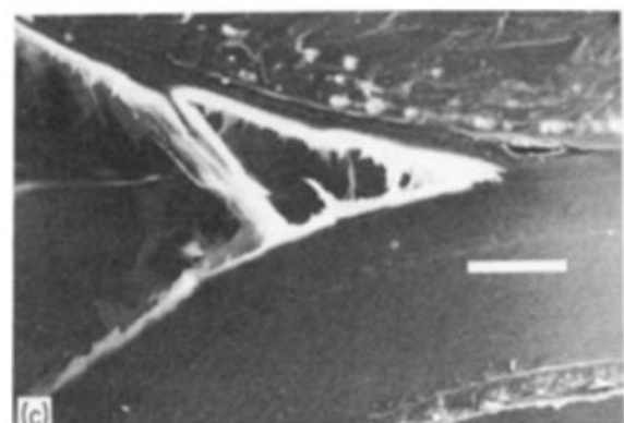
Figure 5 The proposed mechanism for crack advance seen in operation. (a) Opening of a microcrack ahead of the main crack tip and on a plane several micrometres above the latter; (b) stretching of the intervening material to form a ligament bridging the crack; (c) further ligament extension and forward crack growth: note the new microcrack forming near the current main crack tip. All scale bars 30 \mu\text{m} .
